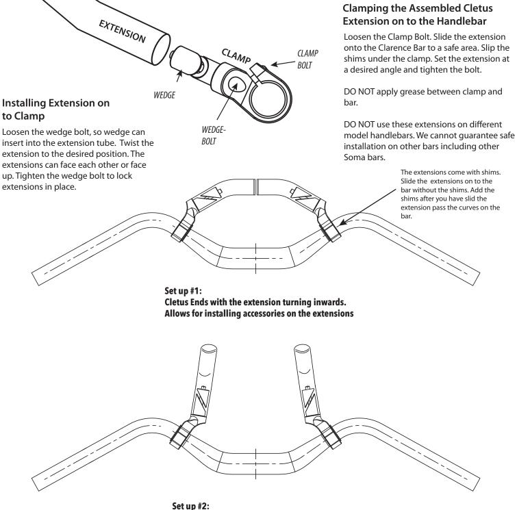
Set up #2: Left and right Cletus Ends swapped to opposite sides - with the extensions rotated upwards. Allows for a more aero ride position.
