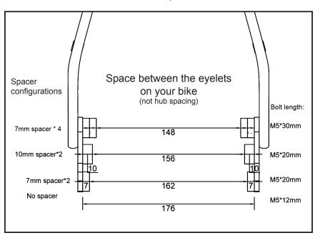
6) Tighten the bolts holding the rack to the upper set of eyelets to about 5 nM.
